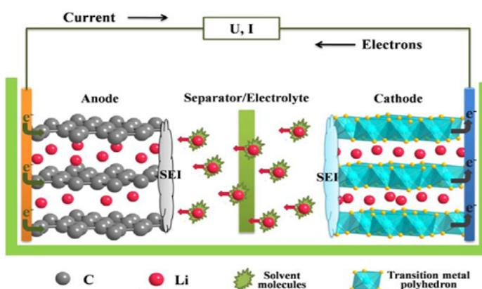
**Fig.1:** Working principle of Li-ion battery
